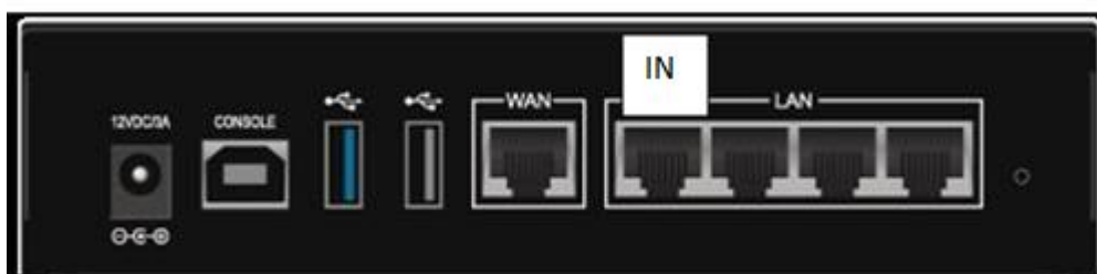
Figure 122: Port IN du Firewall Stormshield SN 160
