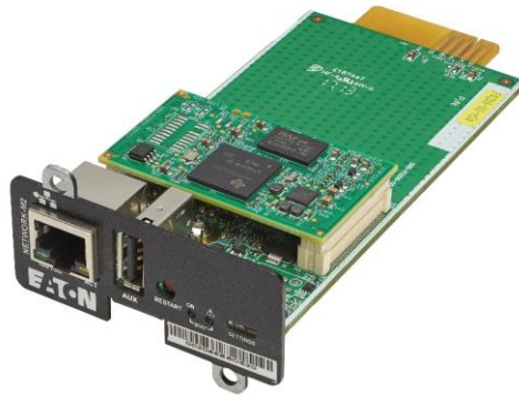
Annexe 2 : Eaton Network-M2
