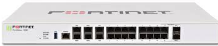
Figure 14 : firewall FortiGate 100E
